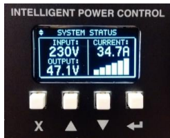
Figure 9: ICM Front Control Interface – System Status Screen
